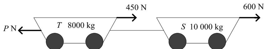
The acceleration of the system is  $0.3\text{ ms}^{-2}$  in the direction of the pulling force of magnitude  $P$ .
