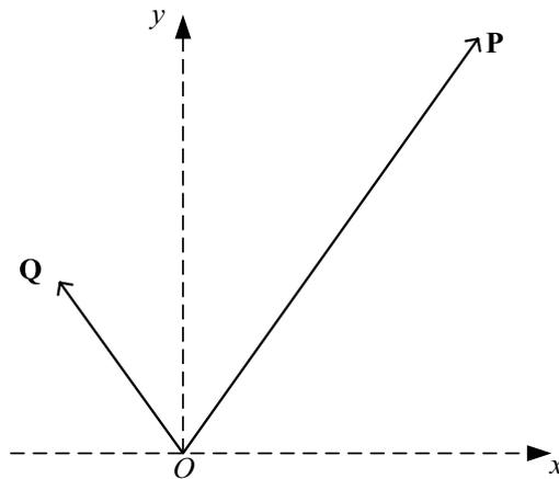
The diagram shows two horizontal forces **P** and **Q** acting at the origin *O* of rectangular coordinates *Oxy*. The components of **P** in the *x*- and *y*-directions are 12 N and 17 N respectively. The components of **Q** in the *x*- and *y*-directions are  $-5$  N and 7 N respectively.
