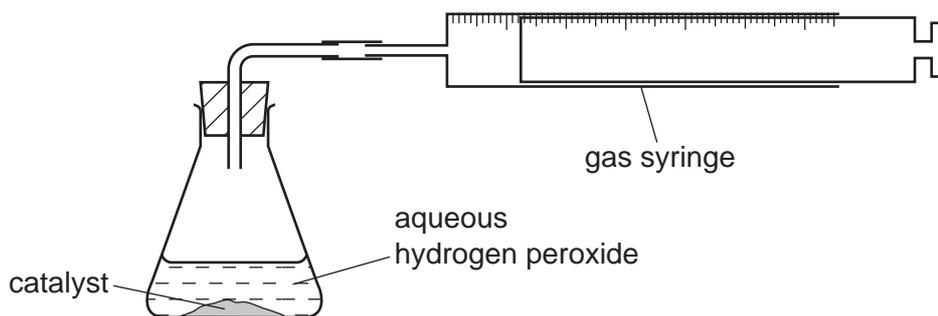
The gas syringe diagrams show the volume of oxygen formed every 30 seconds in each experiment.
